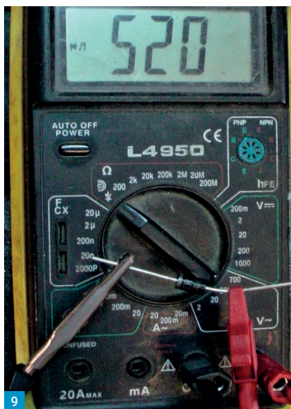
Fig. 8: Measuring current through the 'rectifier' diode. Fig. 9: A silicon diode under test with a digital meter. Fig. 10: Current flow under forward bias. Fig. 11: Current flowing under reverse bias.
